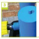
Remove collar Push 6mm pipe through collar and attach to AQUAvalve nozzle Rescrew collar - DON'T overturn... when you feel it grip **STOP**
